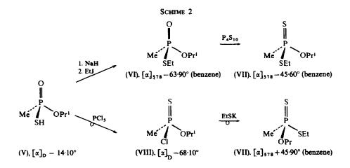
that the reaction of the (-)ester VI with  $P_4S_{10}$  occurs with predominant retention of configuration at phosphorus.
